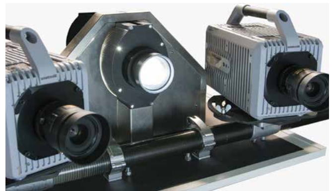
Sensor head of gobo measurement system developed by Fraunhofer IOF
